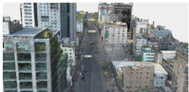
3D models of urban sites are generated using drone aerial photography, and the models are used to determine where to acquire land and where to locate underground train stations.
