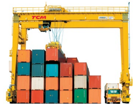
Rubber-tired gantry crane
