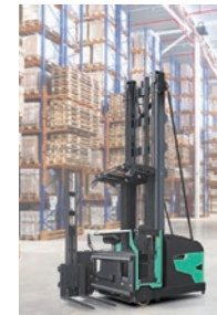
Lateral stacking truck
