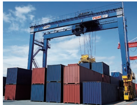
Rubber-tired gantry crane
