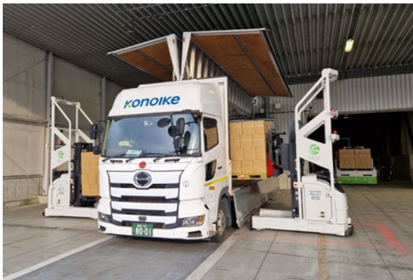
Automated truck loading using PLATTER AUTO
