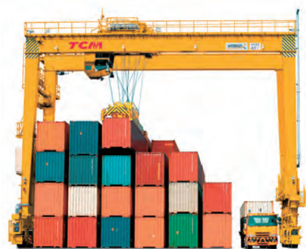
Rubber-tired gantry crane
