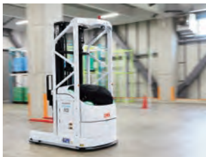
PLATTER Auto H type automated guided forklift
