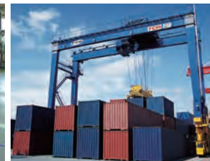
Rubber-tired gantry crane
