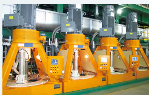
Centrifuge for sugar refining (used to separate sugar crystals) We have delivered more than 1,000 sets worldwide.
