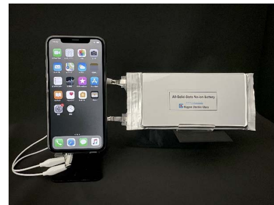
Smartphone operation experiment with an all-solid-state Na-ion secondary battery
