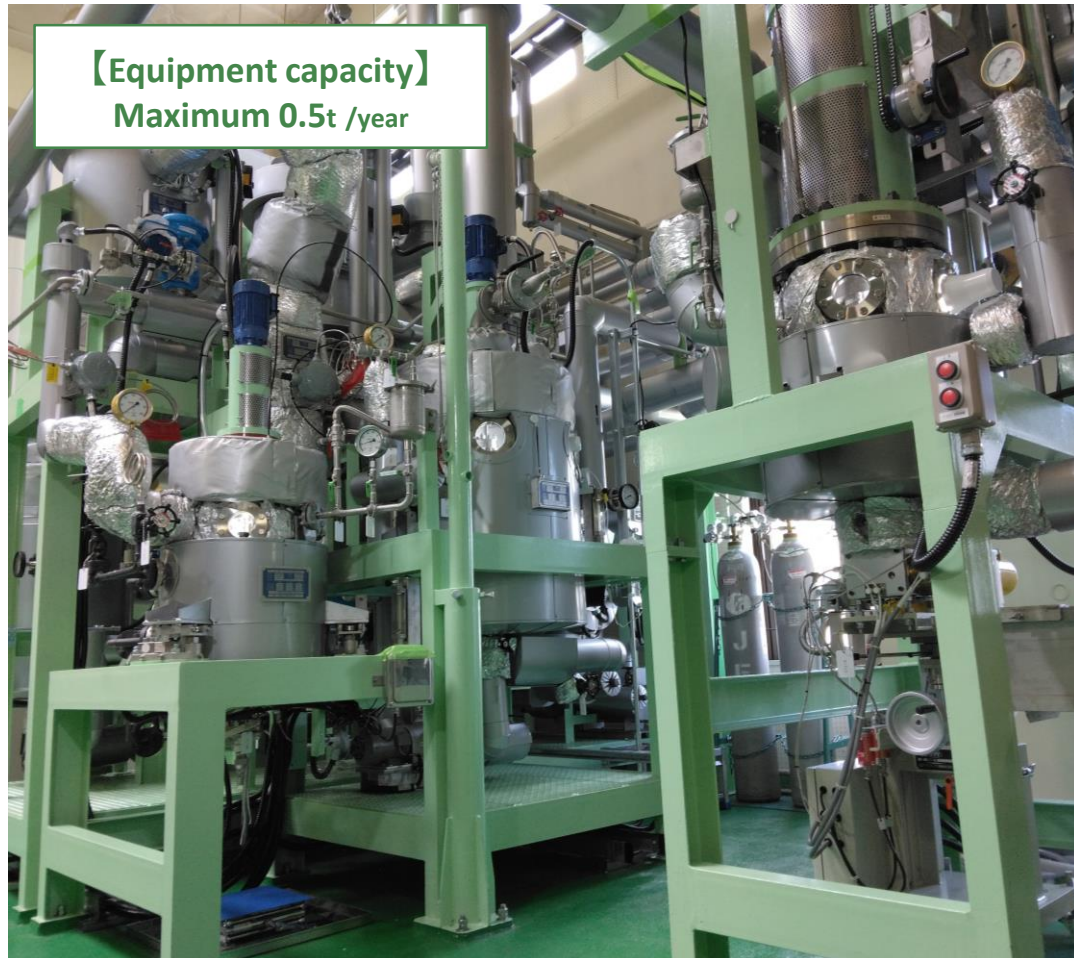
Bench Plant for the synthesis of wood-derived polylactic acid
