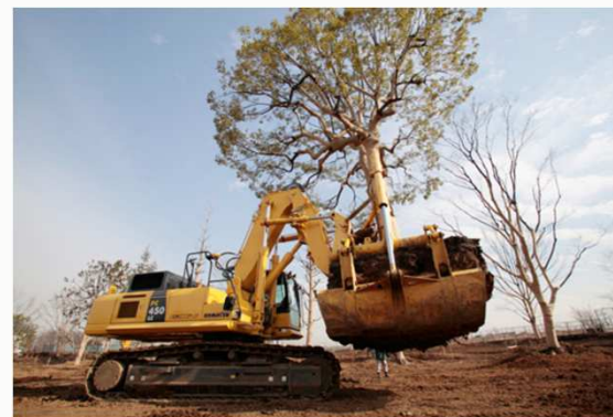
Transplanting work using a TPM machine
