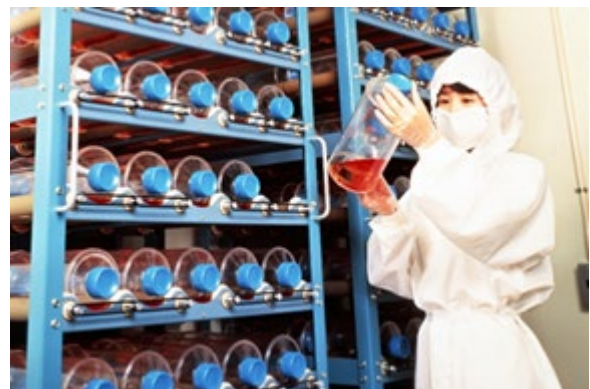
Roller Bottle System Developed by Kirin to scale-up EPO Production
