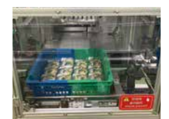
Automated crate removal system for prepared food products (Introduced in October 2024)
