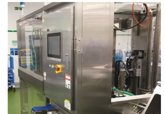
Automated filling machine for onigiri rice ball containers
