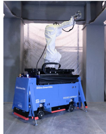
Extended outriggers Robo-Spray II
