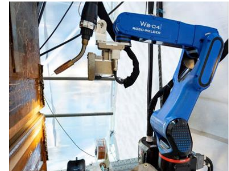
"Robo-Welder" welding steel columns
