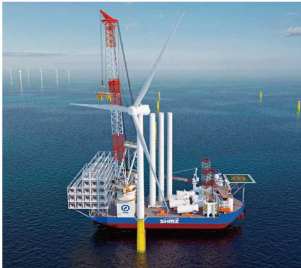
Exterior appearance of self-propelled SEP vessel to be constructed (installing wind turbine blades)
