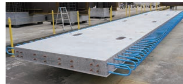
Completed PC road bridge slab
