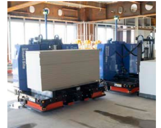
Robo-Carrier improves conveyance efficiency
