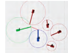
Display showing operation of six crawler cranes (Capable of displaying a bird's-eye view of the entire cranes from above)
