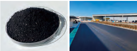
Left: Biochar mixed with asphalt Right: Application example at NIPPON ROAD Tsuchiura Techno BASE (Tsuchiura City, Ibaraki Prefecture)
