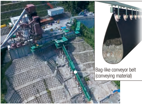
SC premium belt conveyor installation (Ikeda-cho, Imadate-gun, Fukui Prefecture)
