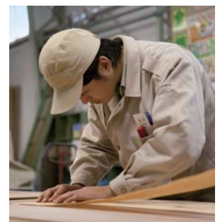
A craftsman (above) covers plywood or flame retardant baseboard with natural wood veneer and another craftsman (left) fashions wood into round wood shapes or large blocks appropriate for their use.
