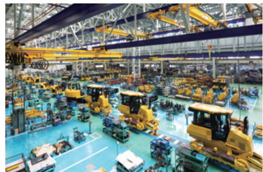
Equipment and pipes are placed in pits along the tracked vehicle assembly line to open up more space for assembly line workers.
