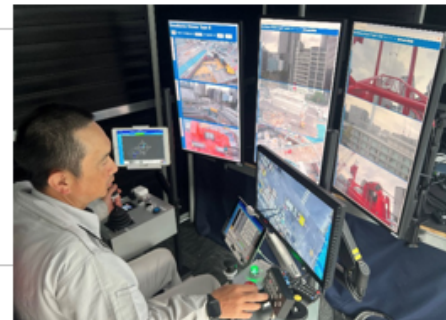
TawaRemos, a remote tower crane control system (jointly developed by Construction RX Consortium)
