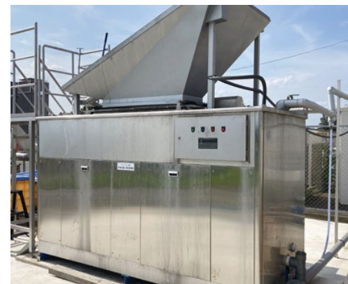
Equipment for processing food waste into fertilizer raw materials (Kodama Plant of Joyous Foods)
