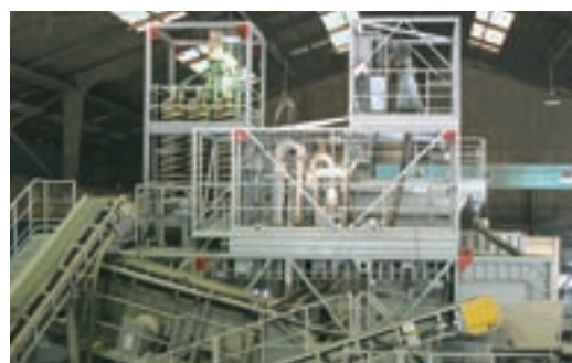
A stationary soil treatment plant (at Kawasaki Office)
